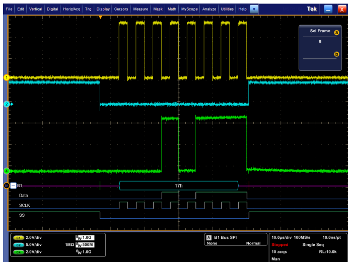
FastFrame™ - User selectable memory segments allow for efficient memory management with time stamped capture of SPI bus data along with analysis of serial bus decoding on multiple data packets. Frames 1, 2, and 9 are shown here.
